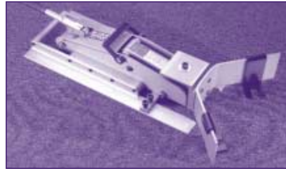
Hydraulic lift with adjustable custom clips for different panel manufacturers.
